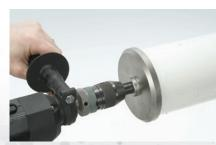
Driven off an adaptor in a power tool, the Soil Pipe Chamfering Tool is designed to remove the burr from around soil pipes to prevent seals being pushed out of fittings when assembled. The carbide grit section chamfers your pipe in seconds and also provides excellent tool durability
